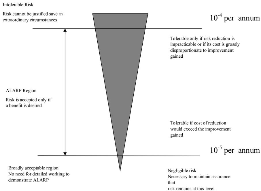
Figure 3.4 ALARP, as low as reasonably practicable, based on Wells (1996) and Melchers (1993) The upper line (intolerable risk) is set at  $10^{-4}$  per annum and the lower one, defining the broadly acceptable region, is set at  $10^{-5}$  per annum for the present application.
