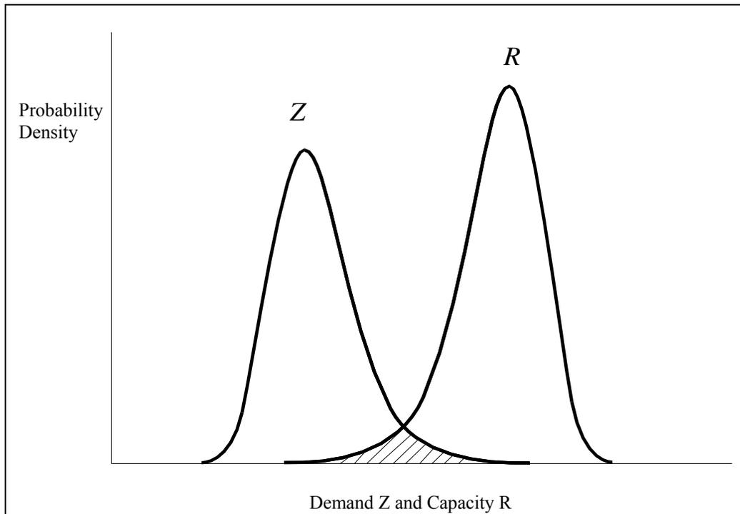
Figure 3.3. System demand and capacity. Overlap area indicates possible failure.
