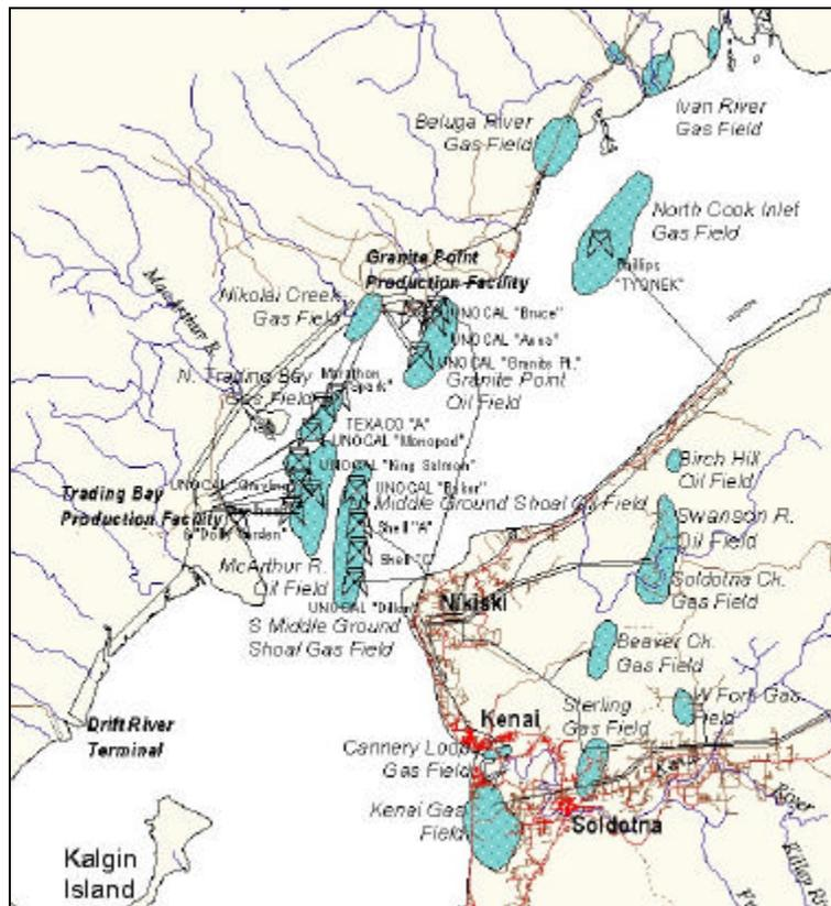
Figure 10.3. Map of Cook Inlet basin and oil facilities. Oil and gas fields are outlined in blue; pipelines are also indicated. An oil refinery is located at Nikiski. (From Cook Inlet Keeper, 2003).
